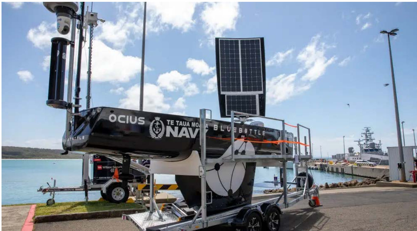
Image: The Bluebottle can run on solar, wind, or wave power, utilizing a rigid sail to provide wind propulsion and photo-electric cells on the sail to drive its motor. Photo: Royal New Zealand Navy
